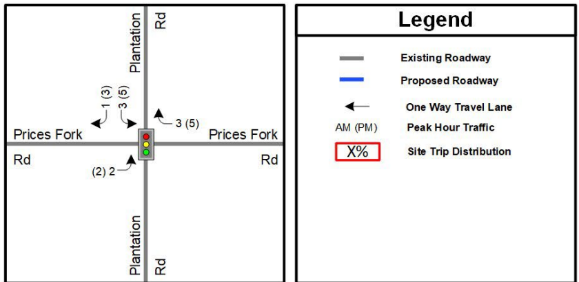
Figure 7: Site Trip Distribution and Assignment
