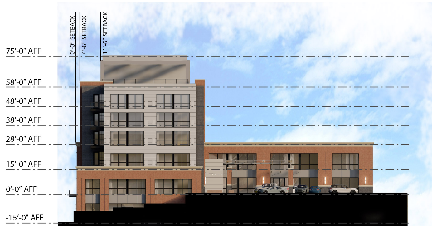
BUILDING ELEVATION - NORTHEAST
