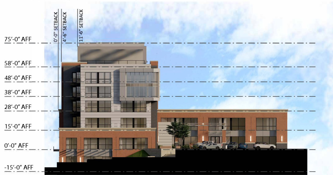
BUILDING ELEVATION - NORTHEAST
