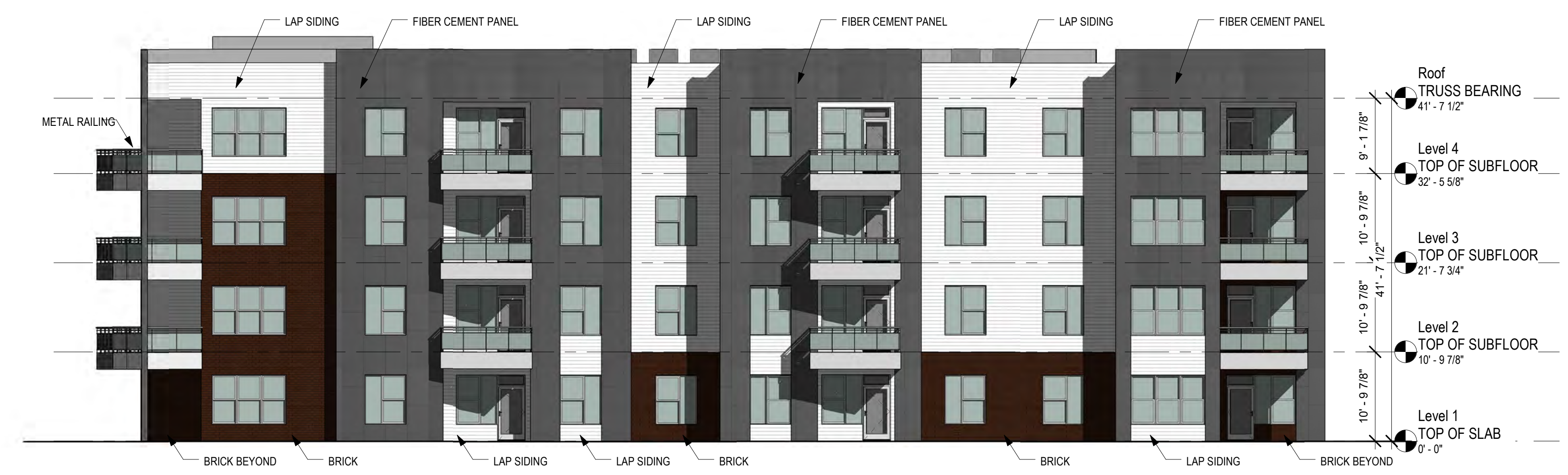
2 BUILDING B - WEST ELEVATION 3/32" = 1'-0"
