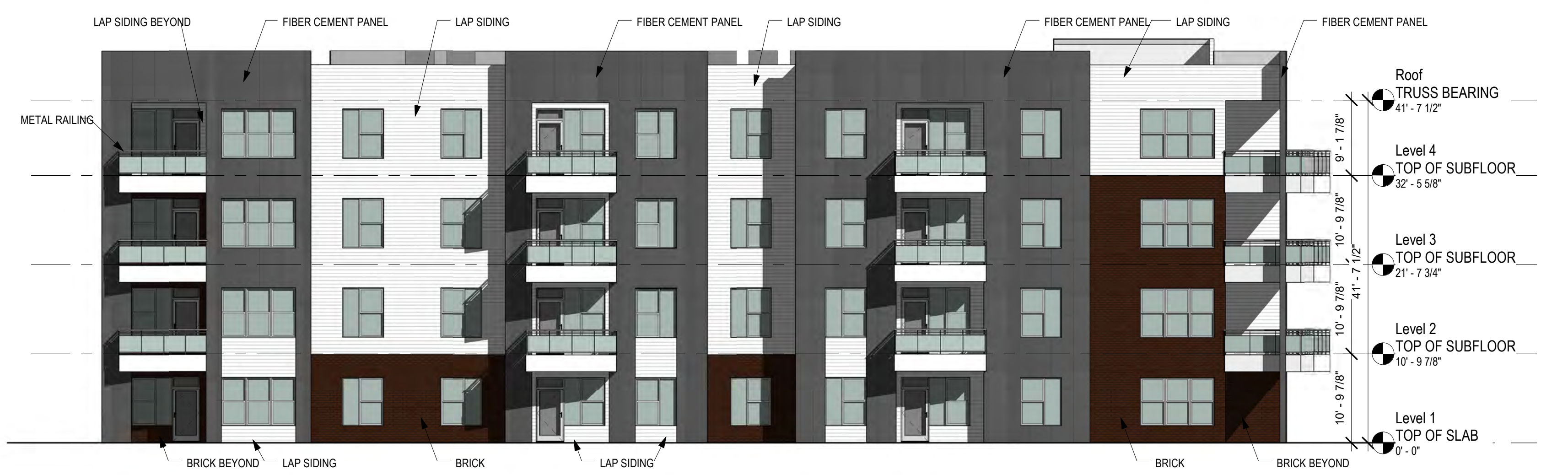
1 BUILDING B - EAST ELEVATION 3/32" = 1'-0"
