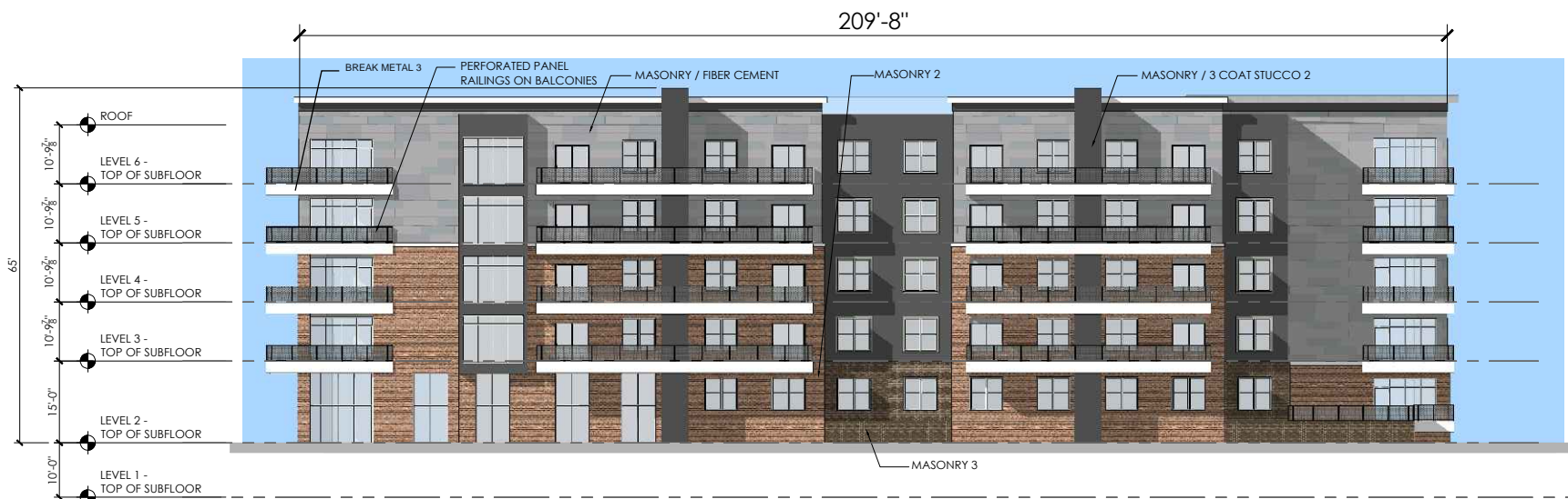
② DC5 BUILDING ELEVATION - PARK VIEW SCALE: 1/8"=1'-0"
