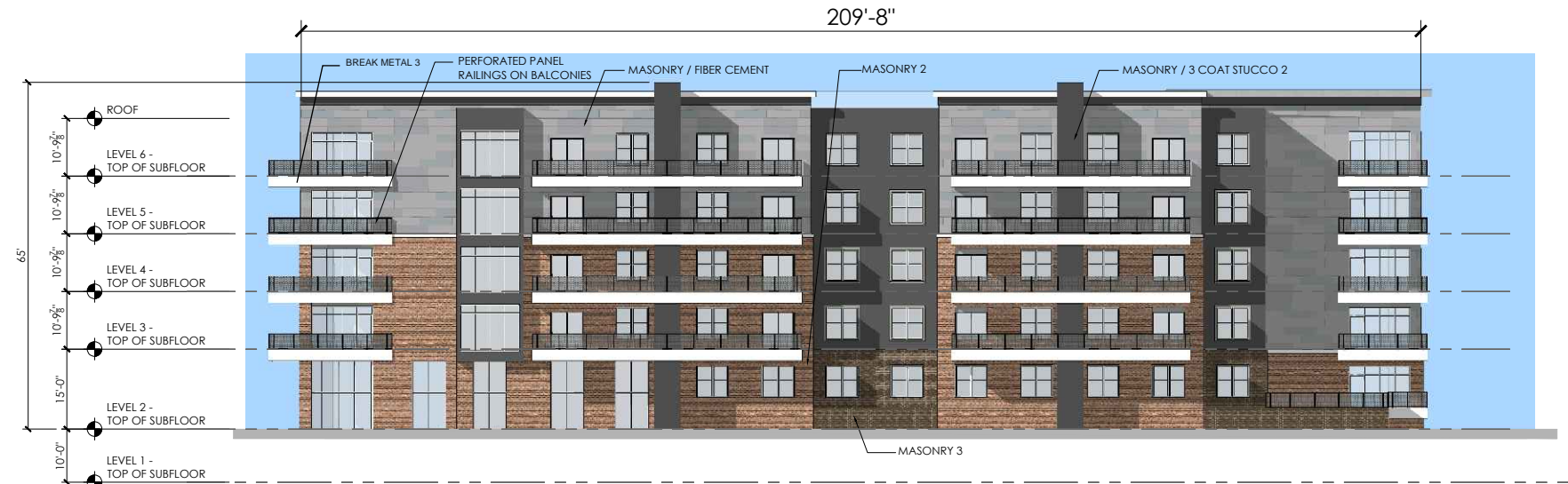
② DC5 BUILDING ELEVATION - PARK VIEW SCALE: 1/8"=1'-0"
